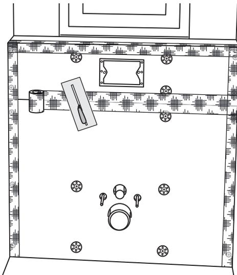
5) Seal all joints and edges with glass fibre tape (e.g. JACKOBOARD® glass fibre tape).
