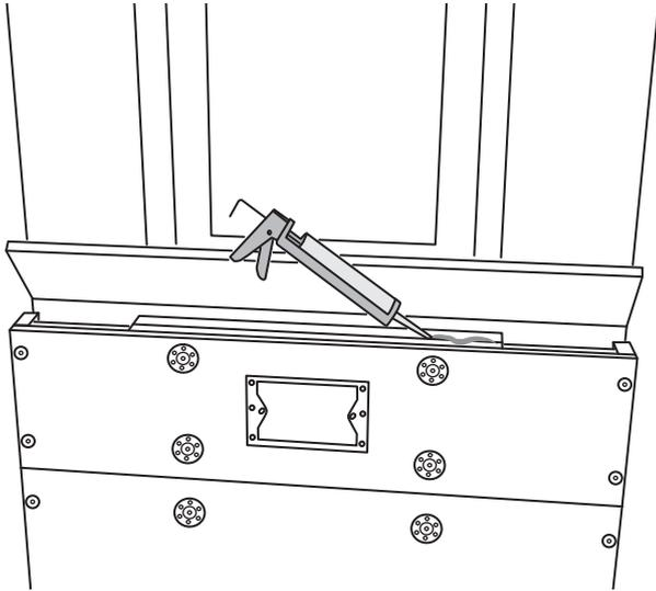
4) Cut out the cover and either bolt it into place or use PU assembly adhesive (e.g. JACKODUR® assembly adhesive) to glue it into place.
